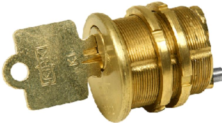
The Type CN22 is a threaded cylinder interlock, commonly installed on circuit breaker interlocking kits. The cam on the back of the cylinder is made to interact with existing linkage on your equipment. The key is trapped or released according to the position of the cam. The CN22 can be linked to other CN22s with the proper bracketry.
